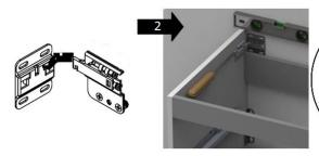
2 Tighten the brackets on the unit so that the furniture fits to the wall and adjust the levels
