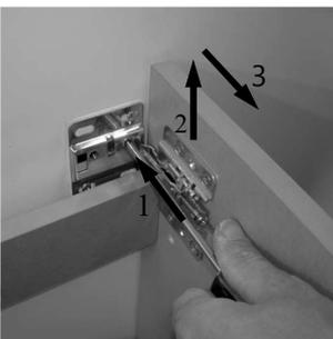
Push inwards with a screwdriver on the tongue, shaped flap, as shown in picture whilst lifting and pulling unit towards you.
