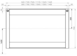
All dimensions are in mm. Recommended height 1600 mm to the centre of the mirror.
