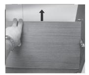
It is necessary to position the rear in the opposite direction to that of step 3 so it win sit on the bottom of the unit.
