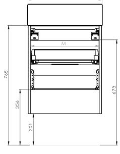
All dimensions are in mm. The dimensions are given to the bottom of the wall plate.
