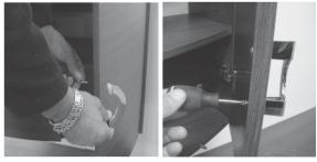
Fix the handle «BP»with the screws «0227» The fascia is pre-drilled
