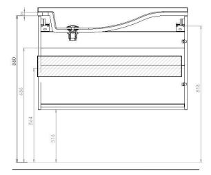
All dimensions are in mm. The dimensions are given to the bottom of the wall plate.
