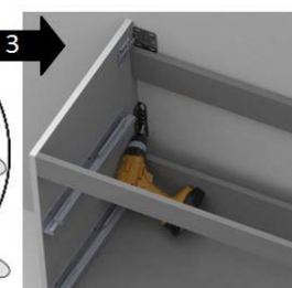
3 Fix the brackets to the wall (screws and wall plug not provided)
