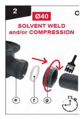
2- Connect the waste body (e) to the waste pipe while respecting a slope of 2%, depending on the model: Ø40 outlet to compression fit and/or glue (ABS/PVC solvent glue), Ø40 UK outlet to compression fit and/or solvent glue (ABS/PVC glue).
