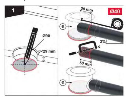
1- Pre-positioning the shower tray. Mark the location of the waste body (e) under the tray with the pencil. Remove the tray. Define the lengh and location of the waste pipe.
