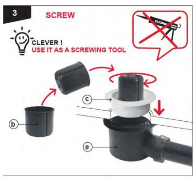
3- Position the tray. Secure the waste body (c) using the flange, use the cup (b) to tighten.
