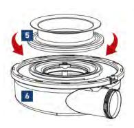
Place the AUTOFIX seal (5) on the drain body (6)
