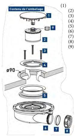
Drain cover (Not Included) Water guard pipe Stainless steel screw M5x40 (x3) Stainless steel clamping plate AUTOFIX double seal Drain body Conical seal Nut 1'1/2 Blanking plug
