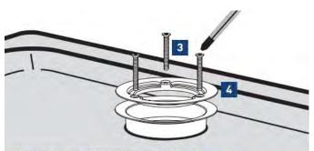
Tighten the stainless steel plate (4) on the drain body (6) with the 3 screws (3)
