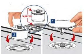
Place the water guard tube (2), position it by aligning the 2 marks (white raised triangle to orange triangle). Insert the cover (1).
