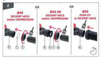
Connect the waste (h) to the outlet pipe ensuring a 2% slope: screw fitting and/or glue fixing (PVC glue) for Ø40 outlet, screw fitting and/or glue fixing (PVC glue) for Ø40 UK outlet, or push-fit fitting or glue fixing (PVC glue) for Ø50 outlet. Ensure to observe the glue drying time indicated.
