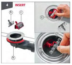
The cartridge (c) then the filter (b) must be inserted into the waste (h). DO NOT THROW AWAY!
