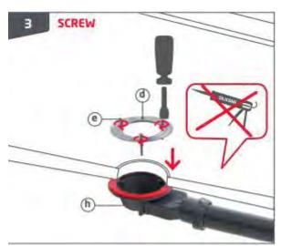
Position the tray. Screw on the metal plate (d) with the screws (e) provided. SILICONE MUST NOT BE USED!
