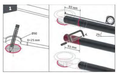
Position the tray as required. Mark the position of the waste under the tray with a pencil. Remove the tray. Define the lenght and position of the outlet pipe.
